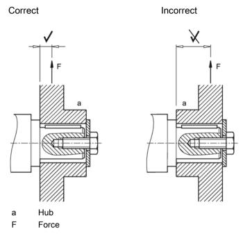
Figure 3-2 Mounting arrangement for low stress on shafts and bearings
