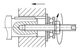
Figure 3-1 Example of a fitting device
