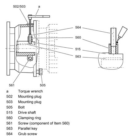
Figure 3-4 Short coupling lantern with clamp connection
