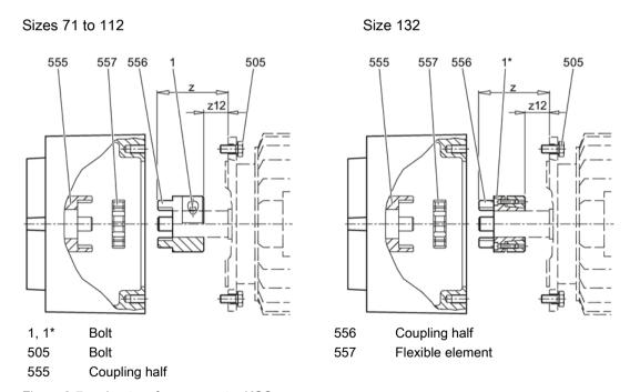
Figure 3-7 Lantern for servomotor KQS
