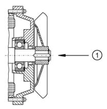
Figure 3-5 Pressure on motor shaft
